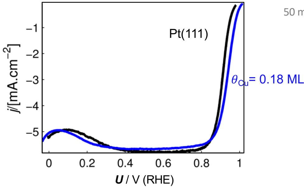
50 mV/s in O<sub>2</sub>-saturated 0.1 M KOH, 1600 RPM
