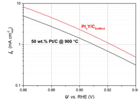
$\text{O}_2\text{-saturated } 0.1 \text{ M HClO}_4, 1600 \text{ RPM } 23^\circ\text{C } 50 \text{ mVs}^{-1}$
