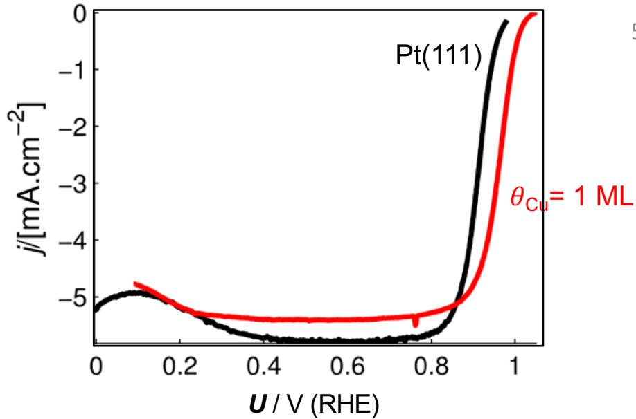
50 mV/s in  $\text{O}_2$ -saturated 0.1 M KOH, 1600 RPM
