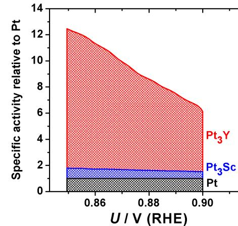
Kinetic current density in O<sub>2</sub>-saturated 0.1 M HClO<sub>4</sub>, 23 °C 20 mV/s, 1600 RPM
