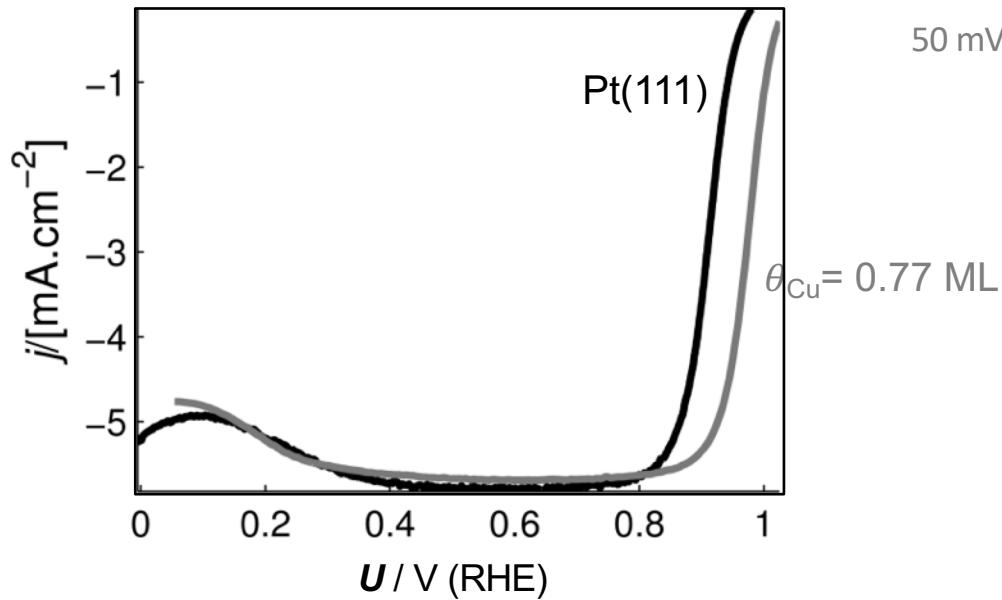
50 mV/s in  $\text{O}_2$ -saturated 0.1 M KOH, 1600 RPM
