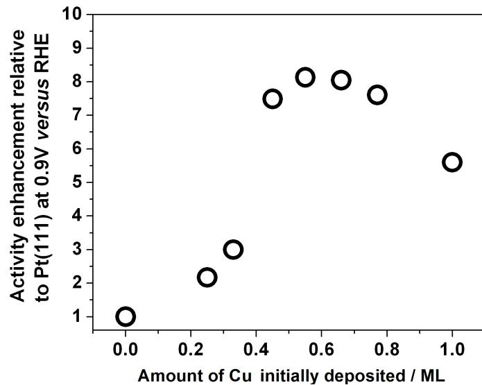
$U = 0.9 \text{ V}$ , 50 mV/s, 1600 RPM in O<sub>2</sub>-saturated 0.1 M HClO<sub>4</sub>
